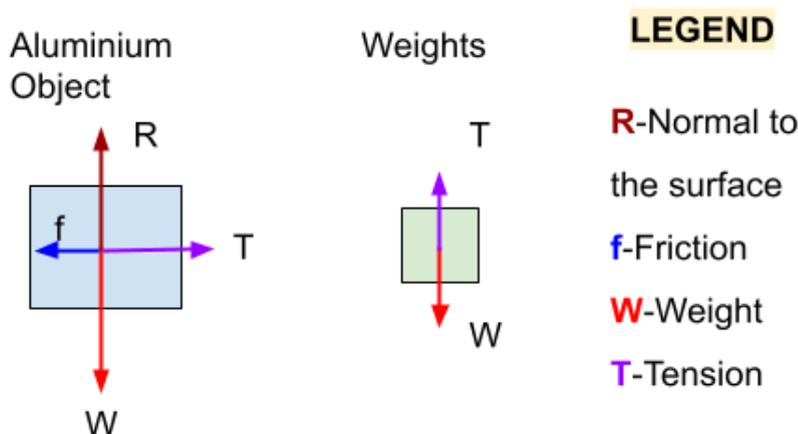
In order to determine the **coefficient of friction**, a free-body diagram of the weights and the aluminium object was made.
